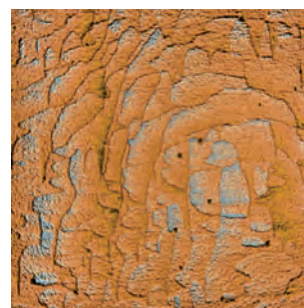
Monolayer steps on the Si surface. Scan size: 5x5 \mu\text{m} . Image courtesy: Dr. Jerry Floro, University of Virginia.
